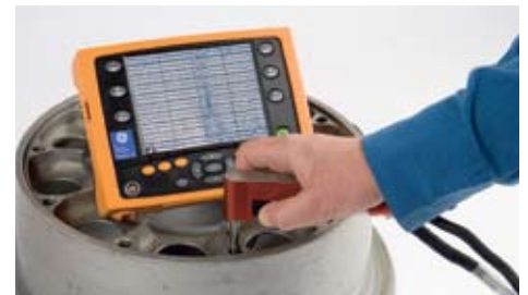
Rotary inspection of aircraft wheel tie bolt holes.
