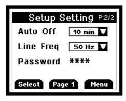
This screen below is used to reset/change password. In the event if uses forget his/her password, 5586 can be used to reset to a new value
