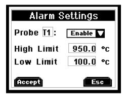
Disable or enable the alarm for individual probe by pressing recall ▲ or log ▼ and F1 to accept. Increase or decrease individual limit by pressing recall ▲ or log ▼.
