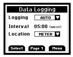
Press recall ▲ or log ▼to choose the logging methods as auto or manual. If it is auto logging, using recall ▲ or log ▼to set time interval. Its range is from 0min to 60min.
