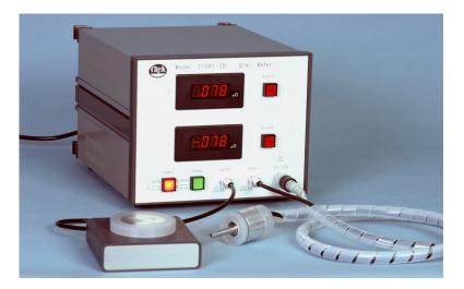
A Q/m analyzer which avoids the creation of measurement errors associated with traditional "blow-off"
